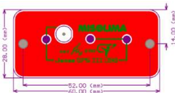
Figure 6. GPS Panel mounting with 3M holes
